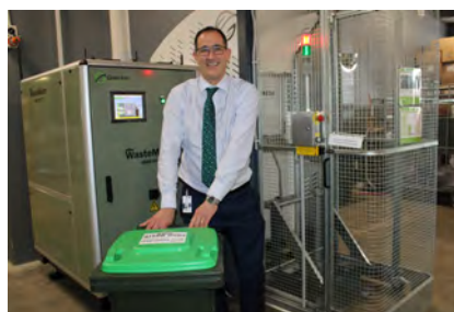
Catering manager Peter Trusler with a food waste recycling system converting leftover food and compostable packaging into biofuel for electricity generation.
